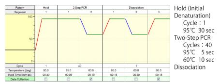
3. After the reaction ends, check the amplification curve and melting curve. Prepare a calibration curve if quantitation is to be performed.
