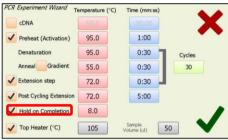
Edit the 'PCR Experiment Wizard' screen. Create new program that note the temperature, the reaction time and number of cycles etc.
