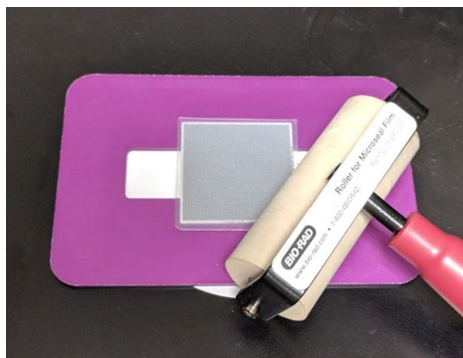
Figure 81. Sealing the chip with film and a film-sealing roller.
