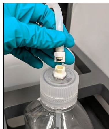
Figure 55. Disconnecting the quick-connect fitting from the wash bottle cap.
