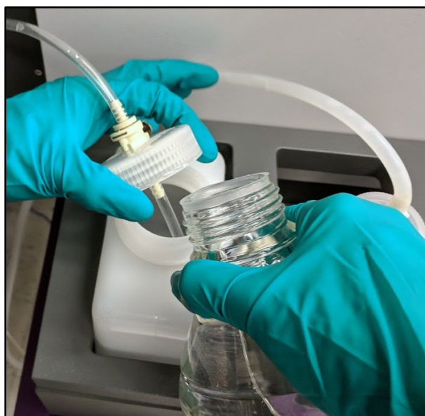
Figure 54. Recommended method of refilling the humidifier reservoir.
