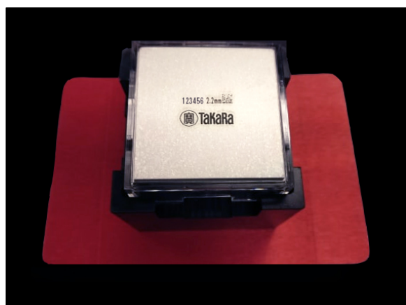
Figure 97. Placing the chip into the collection module.
