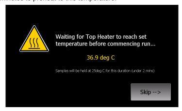
When the run commences the software will automatically proceed to the 'Run' screen. You are not able to modify the profile once a run has commenced.
