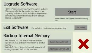
After selecting the software file read the message box and press OK and wait. Upgrade will take up to 1~2 minutes. Once upgrade is complete you can check that the new version is installed by visiting the 'Information' page from the Configure and check the installed software version.
