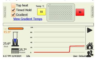
Gradient: If the 'Gradient' checkbox is checked the 'Temp Left' and 'Temp Right' buttons appear and you are able to set different temperatures hat is programmable  $0\sim25^{\circ}\text{C}$  across block width (12wells) for both the left and right sides of the block with a roughly linear thermal gradient presented between the two outer well sides and the predicted well temperatures can be shown by clicking the 'View Gradient Temp' link.
