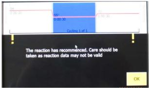
When touch the OK button , start to run the program from the stopped state.
