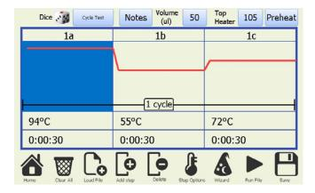
Activating 'Run File' button under the icons will show a profile review page which allows the operator to check over the profile (displayed in text format) before confirming commencement and then click 'Start Run'.
