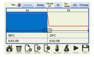
(5) Activating 'Run File' button under the icons will show a profile review page which allows the operator to check over the profile (displayed in text format) before confirming commencement and then click 'Start Run'.
